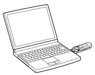
Remove the USB cap and connect the USB connector to a USB connector on your computer. When the remaining battery indication of the display shows:
